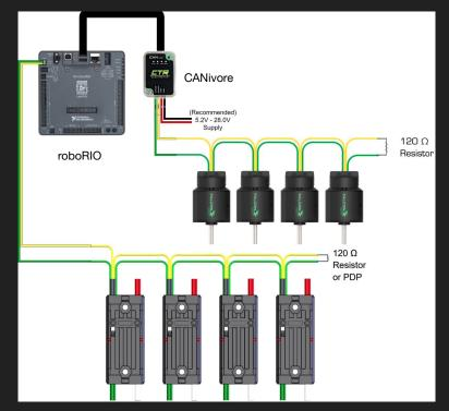
PDH is not shown being connected into the CAN BUS in the above example.
